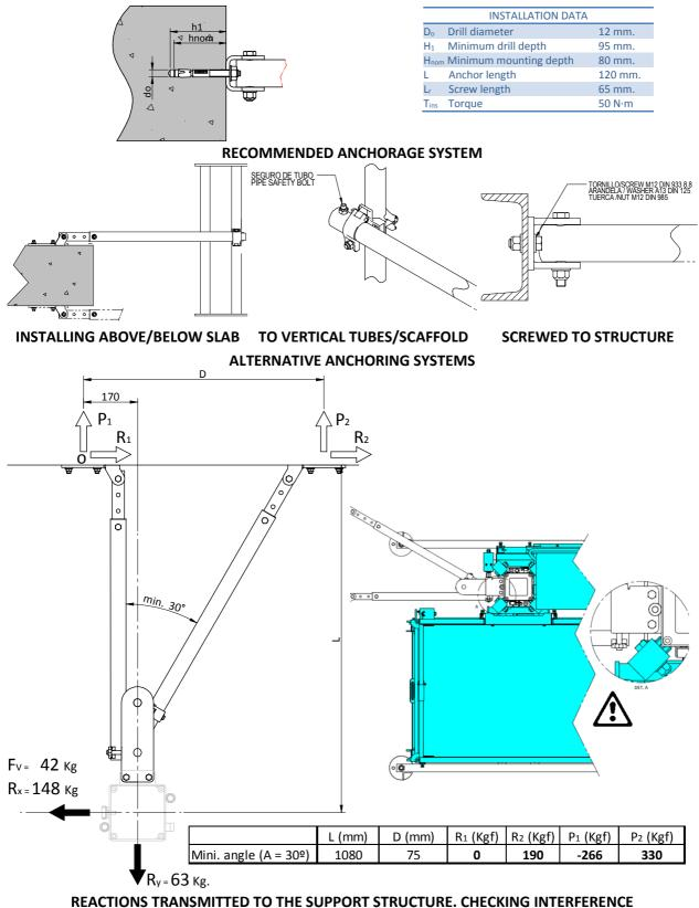
REACTIONS TRANSMITTED TO THE SUPPORT STRUCTURE. CHECKING INTERFERENCE
