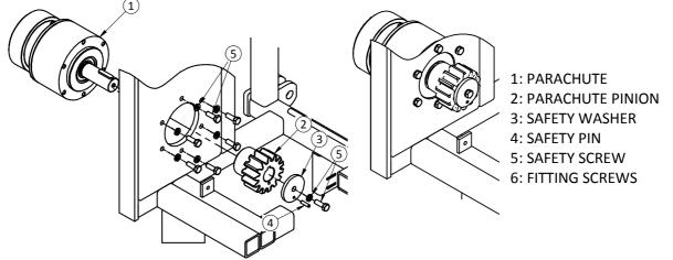
INSTALLING SAFETY UNIT IN TO THE HOIST
