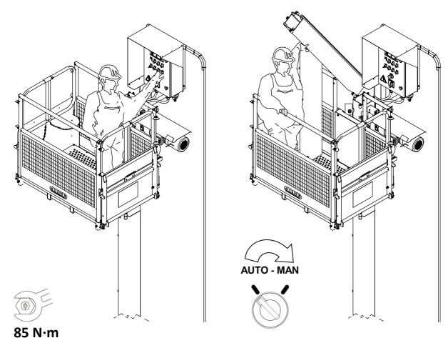
MANUAL ASSEMBLY OF THE MASTS COLUMN
