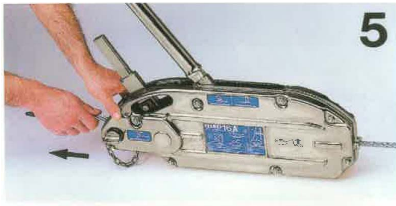
Fig. 2-5 - Pulling the cable out with your hand
