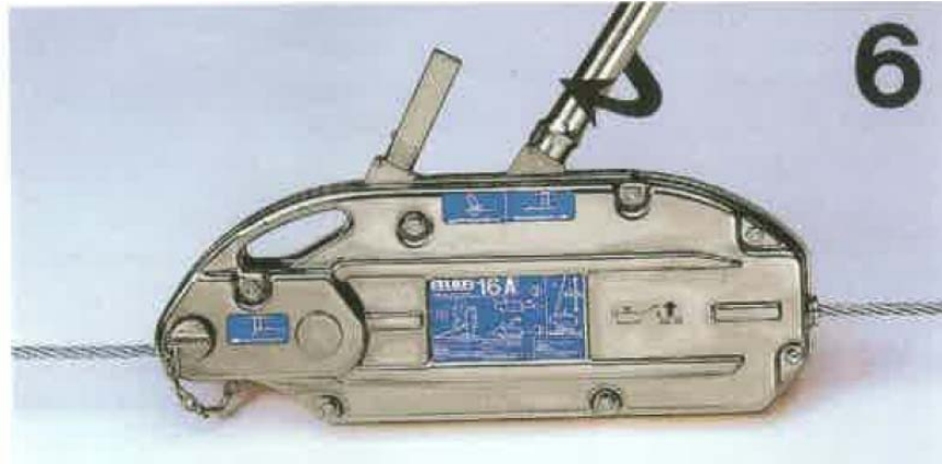
Fig. 2-6 – Placing the lever in position and turning it halfway round to prevent it from coming loose
