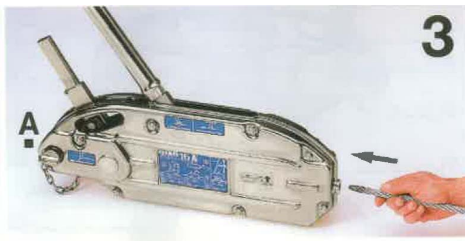
Fig. 2-3 - Introducing the cable
