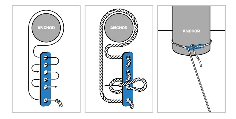
"Knots shall not be used for load bearing end terminations." - ANSI Z-359.1 Section 3.2.7.2.2
