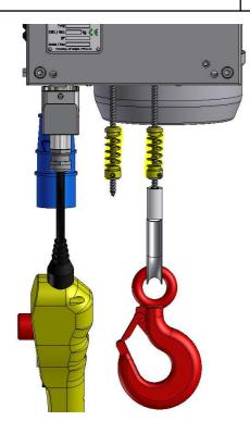
Check the operation of the limit switches of the winch.
