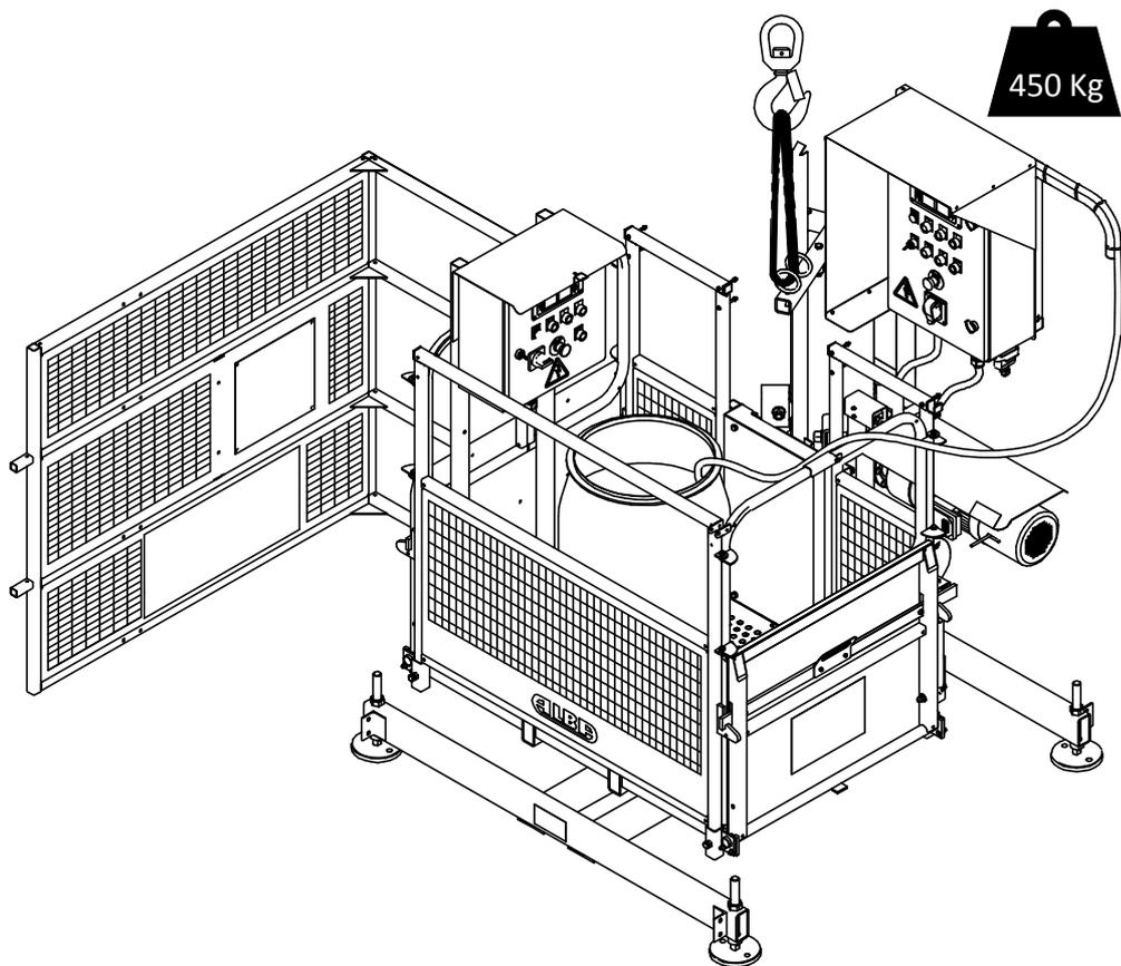
ASSEMBLY OF CAGE. USE A CRANE O FORKLIFT
