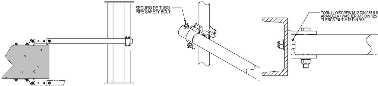
INSTALLING ABOVE/BELOW SLAB TO VERTICAL TUBES/SCAFFOLD SCREWED TO STRUCTURE
