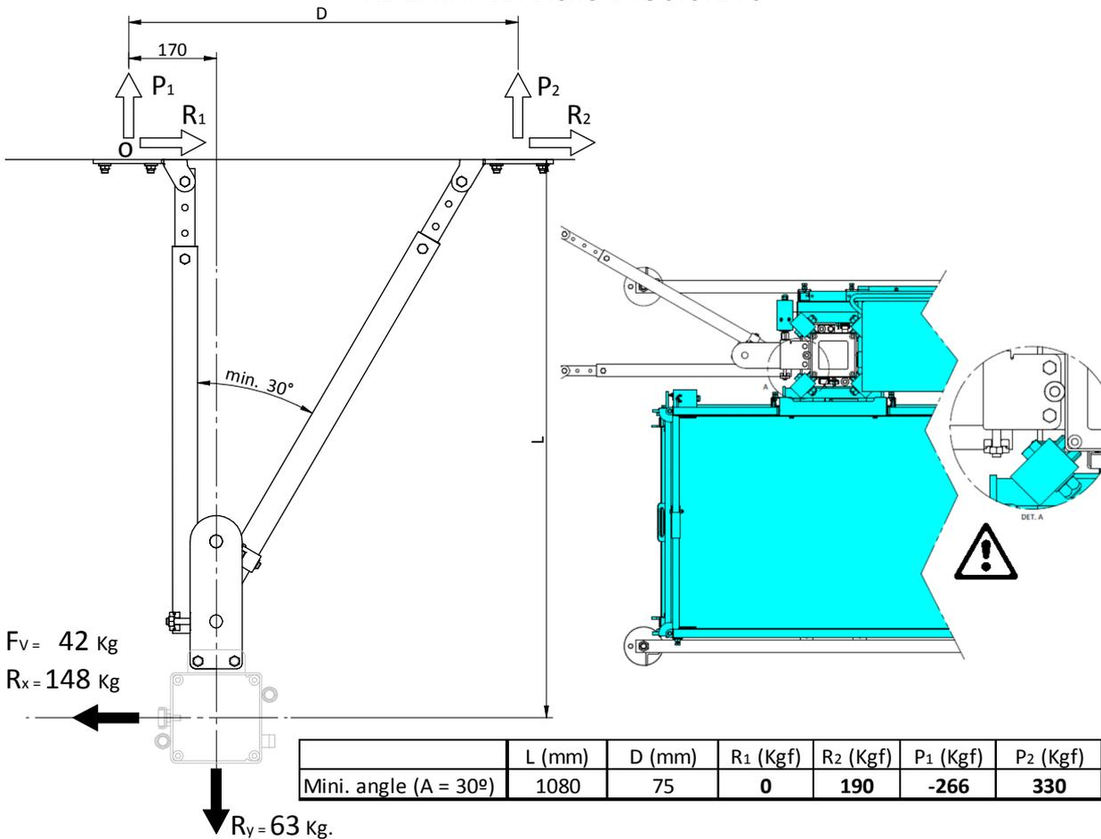
REACTIONS TRANSMITTED TO THE SUPPORT STRUCTURE. CHECKING INTERFERENCE
