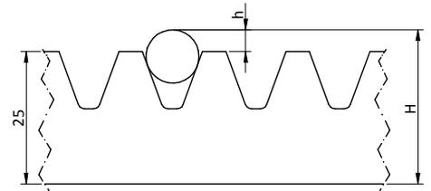
$K_2 \text{ TOOTH} < 21 \text{ mm} \rightarrow$  REPLACE PINION
